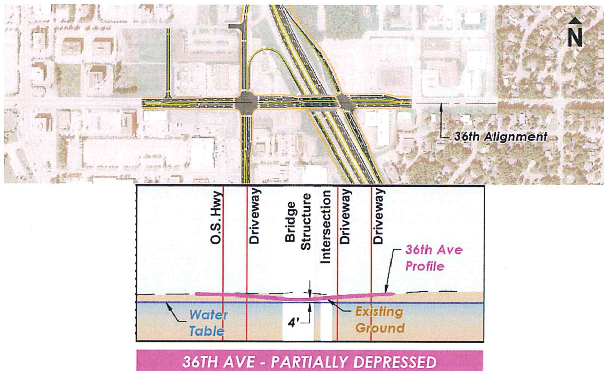
Figure 13: Profile of 36th Avenue partially depressed over a partially elevated Seward Highway
