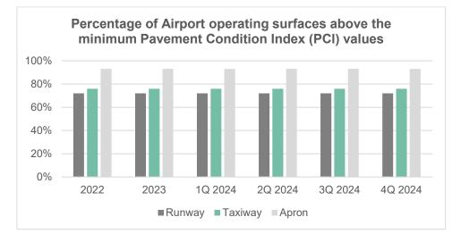
Measures the safety of the airport's pavement maintenance program by reporting the percentage of airport operating surfaces that are above established minimum Pavement Condition Index (PCI) values. (PCI of 70 or higher on Runways, and PCI of 60 or higher on Taxiways, Aprons, and Roadways on a scale of 1 - 100, with 100 being the best condition.)
