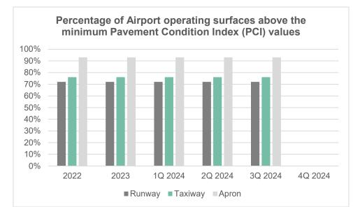
Measures the safety of the airport's pavement maintenance program by reporting the percentage of airport operating surfaces that are above established minimum Pavement Condition Index (PCI) values. (PCI of 70 or higher on Runways, and PCI of 60 or higher on Taxiways, Aprons, and Roadways on a scale of 1 - 100, with 100 being the best condition.)
