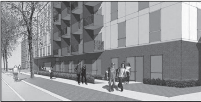
1 CURB CUT 60% OF STREET FRONTAGE OCCUPIED BY GROUND-LEVEL USES PARKING COMPLETELY SCREENED
