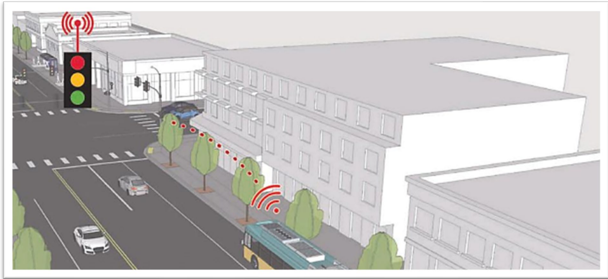
Figure 17 Transit Signal Priority, bus signaling to traffic light
