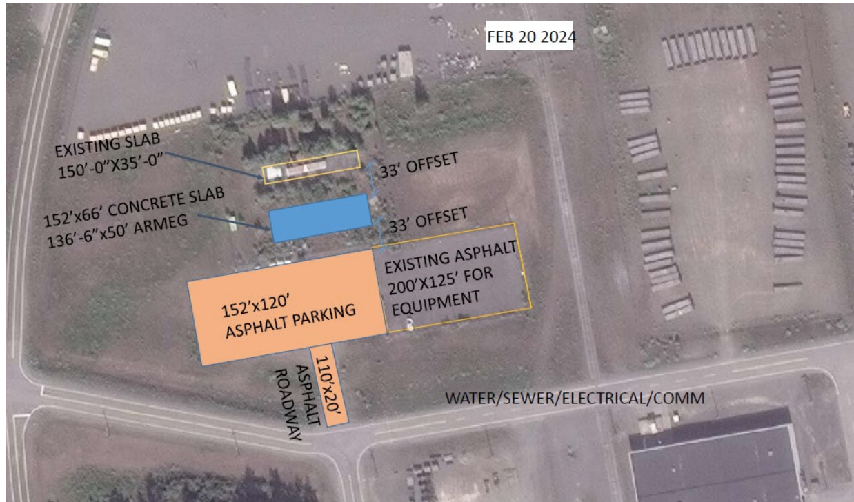
Figure 2. Foundry lot layout and current conditions.
