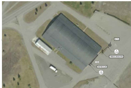
Figure 12. Slab & trench plan Bldg 8326
