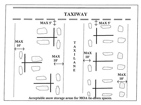
Typically, after a snow fall, Airport Maintenance will plow the taxilane into a berm along the center of the taxilane. The idea is to provide access so airplane owners can drive to their aircraft (sweep off the wings). It may be a couple of days before Airport Maintenance comes back to remove the berm along the center of taxilane.
