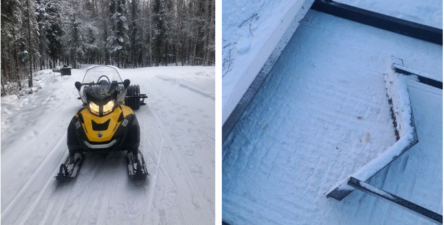
Figure 3: Snow Machine with a roller on the top left. A Colorado attachment, also behind a snow machine, on the right.
