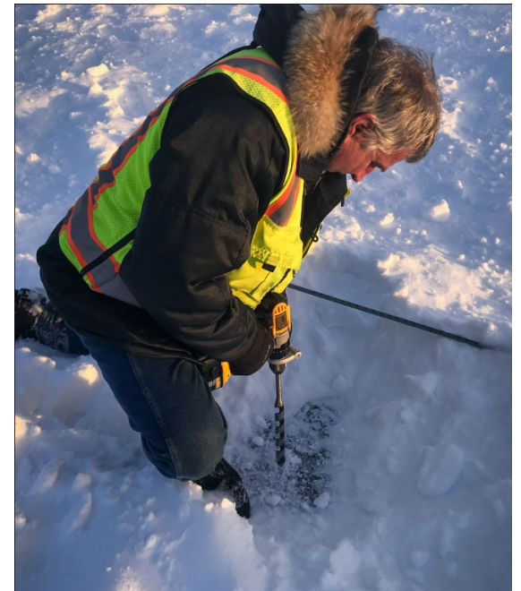
Photos (top to bottom): Top: Snow machine with a Ginsu attachment grooming and “setting track.” Bottom: Maintenance drilling ice on Westchester Lagoon to measure the depth of ice.
