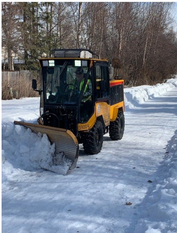
Figure 2: Trackless equipment on top with blower attachment, and on bottom with plow attachment clarifying the edges of an already blown multi-use pathway.
