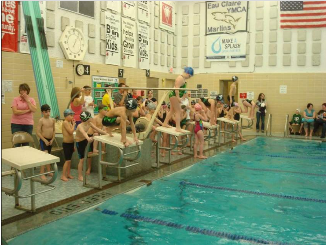
Figure 25- a YMCA has a concrete mounted 1 meter stand. Note how the standard hand rails protrude. The bartlett Design allows the front portion of these railings to be removed for added swimmer safety.
