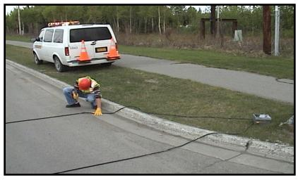
Data Technicians assemble volume study using pressureactivated tubing attached to a digital vehicle counter.
